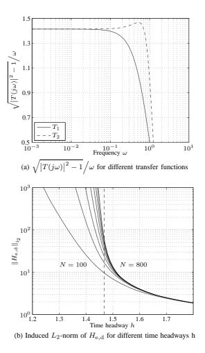
*Example 1 (Infimal Time Headway*  $h_0$ ): In order to find the infimal time headway  $h_0$ , the maximum over all frequencies of  $(|T(j\omega)|^2 - 1)/\omega^2$  must be evaluated. For  $T_1(s) = \frac{s+1}{s^2+s+1}$  the maximum is achieved at  $\omega = 0$  and
