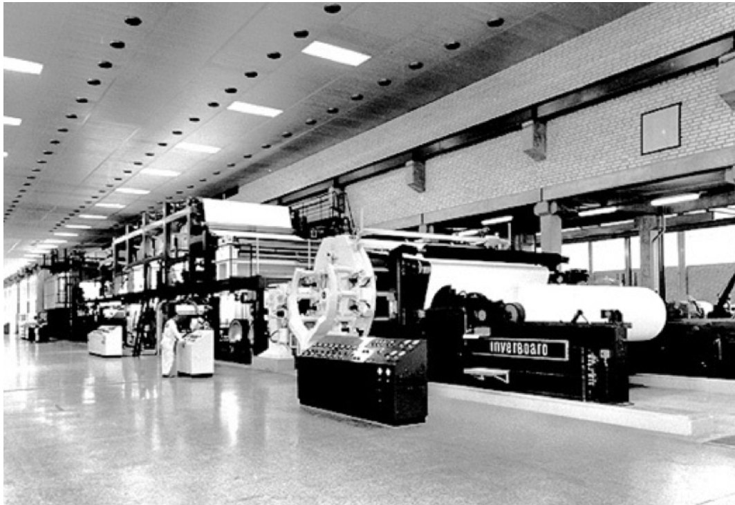
Figure S3. Iggesund Paperboard's first cardboard machine called KM1 and is still in use, but since the photo was taken in 1968, it has been rebuilt several times. The photo is taken so that you see the reeling of the cardboard and in the middle of the picture you see the coating stations. At the far left of the picture, the drying unit of the cardboard machine is visible.
